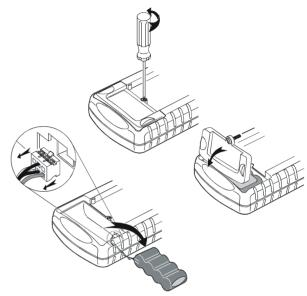
Figure 2-2. Replacing the Battery Pack
