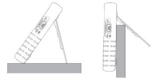
Figure 3-1. Using the Tilt Stand
