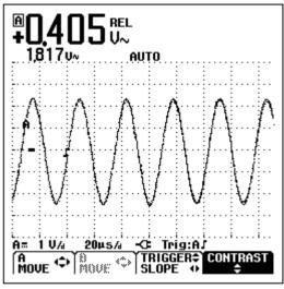
Figure 1-9. Making a Relative Measurement
