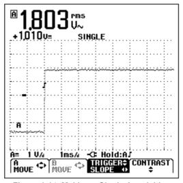
Figure 1-14. Making a Single Acquisition
