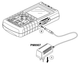
Figure 2-1. Charging the Battery Pack
