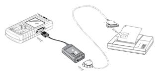
Figure 1-23. Connecting a Parallel Printer
