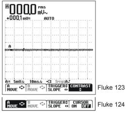
Figure 1-2. The Screen After Reset
