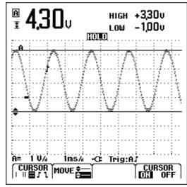
Figure 1-19. Voltage Measurement with Cursors
