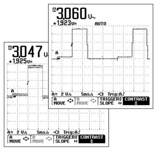
Figure 1-11. Smoothing the Waveform
