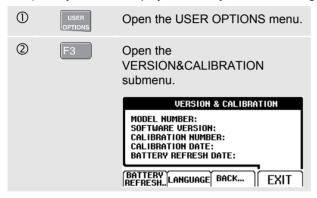
The screen gives you information about the model number with software version, the calibration number with latest calibration date, and the latest battery refresh date.
