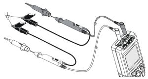
Figure 3-2. Grounding with Short Ground Lead
