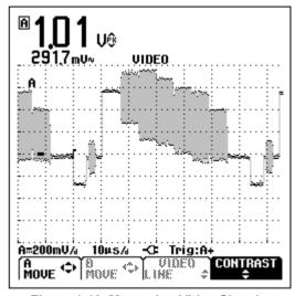
Figure 1-18. Measuring Video Signals
