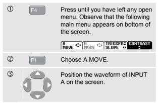
Waveform positioning is demonstrated in Figure 1-10.
