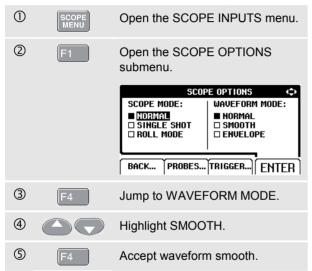
You can use waveform smooth to suppress noise without loss of bandwidth. Waveform samples with and without smoothing are shown in Figure 1-11.
