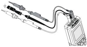
Figure 3-3. Grounding with Unshielded Ground Lead
