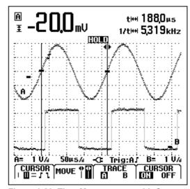
Figure 1-20. Time Measurement with Cursors
