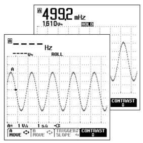
Figure 1-15. Recording Waveforms over Longer
