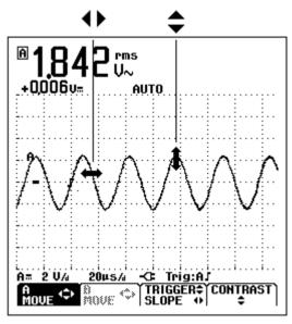
Figure 1-10. Positioning the Waveform
