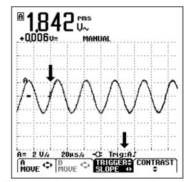
Figure 1-16. Screen with all Trigger Information
