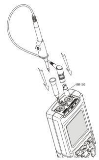
Figure 2-3. Adjusting Scope Probes
