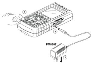
Figure 1-1. Powering the Test Tool
